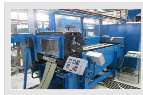
Continuous pasting production line
